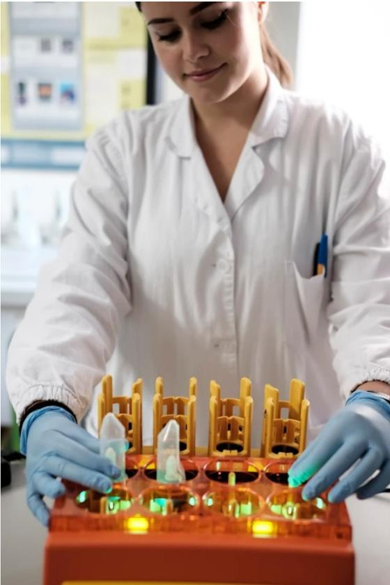
The researcher is inserting a plastic tube containing a suspension of human cells in a centrifuge. The centrifugation utilizes an applied centrifugal force field to separate the cells from the medium in which they were grown.
